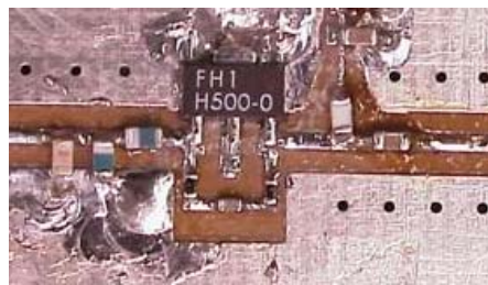
Circuit Board Material: .014” Getek ML200DSS ( \epsilon_r = 4.2 ), 1 oz copper. The main microstrip line has a line impedance of 50 \Omega .
